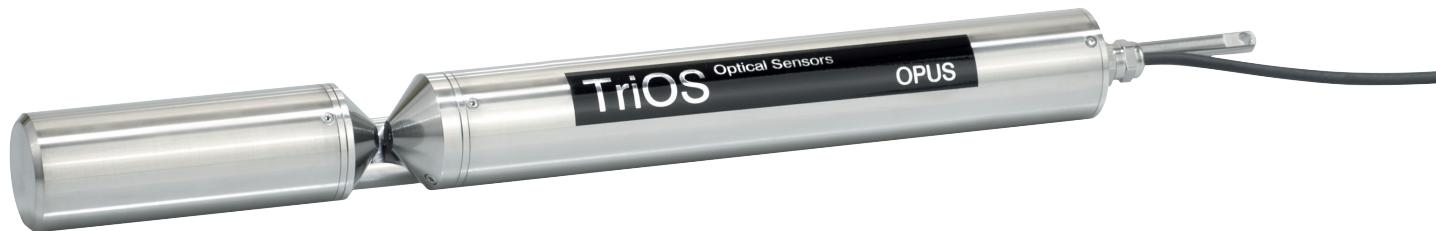
OPUS is the new generation of spectral sensors for online measurement of nitrogen and carbon compounds. Through the analysis of a full spectrum, OPUS is able to deliver reliable readings for  $\text{NO}_3\text{-N}$ ,  $\text{NO}_2\text{-N}$ , organic ingredients (CODeq, BODeq, DOCeq, TOCeq), and a number of other parameters.
