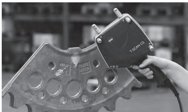
ZEISS T-SCAN:用手持式激光扫描仪快速、直观的捕获三维数据
