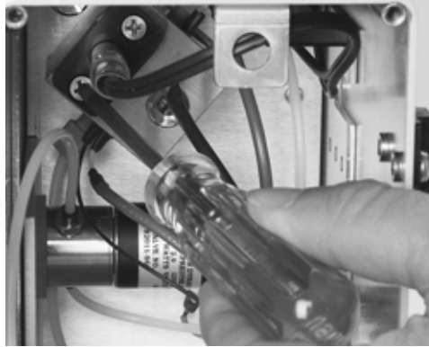
Fig 13-7 : Loosening the UV Lamp Bracket
