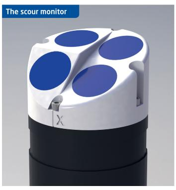
The Scour Monitor head, showing the four transducer arrangement. The instrument has no protruding parts, making mounting arrangements less susceptible to damage.
