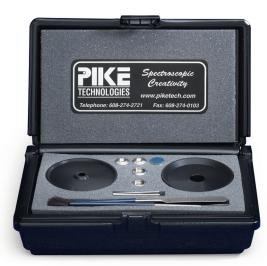
The Sample Preparation Kit makes the handling of powder samples for diffuse reflectance sampling easy. It includes a round mounting base and a matching tray with an opening which accommodates sampling cups. The cup is placed in the assembly and overfilled with sample, and then excess powder is leveled-off with a spatula. The overflow is retained on the tray and can be easily returned to the sample container or disposed.
