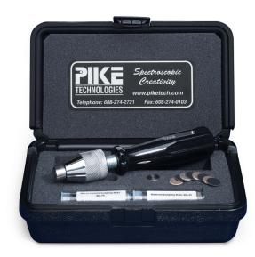
The Abrasion Sampling Kit consists of an abrasion disk holder and a set of silicone carbide (SiC) and diamond disks. Sampling is performed by abrading the surface of the investigated substance with a selected disk. The disk is placed in the accessory and a diffuse reflectance spectrum of the material is collected. This method is particularly useful for the analysis of large painted surfaces (e.g. car panels) and other awkward objects.
