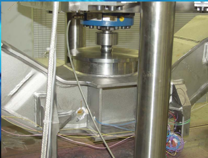
Calibration of a Beam with Strain Gauges
