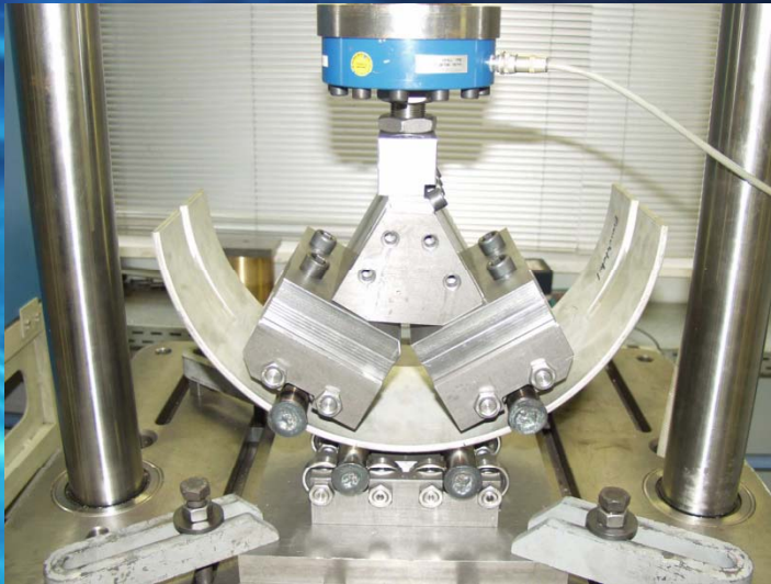
Bending Test of Bearings (Four Point Bending)
