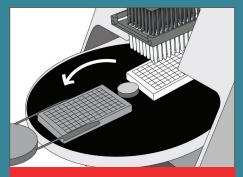
New plate is automatically moved into loading position for further processing, which ensures seamless purification without any delay between steps and use any number of plates
