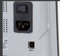
◀ USB connection for temperature probe.
