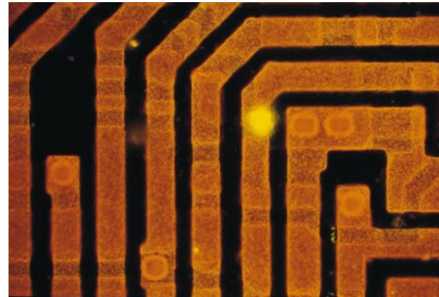
Contamination shown in fluorescence
