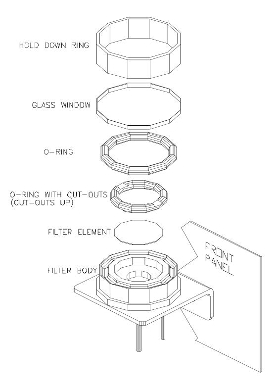
Figure 8-1: Replacing the Particulate Filter
