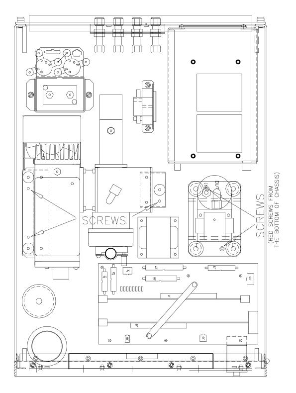
Figure 2-1: Removal of Shipping Screws
