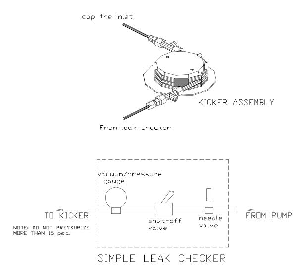
Figure 9-11: Kicker Leak Check
