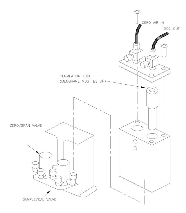
**Figure 6-1: Permeation Tube Installation**
