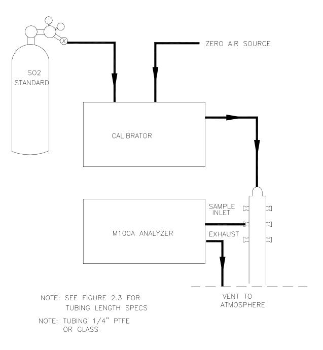
Figure 7-1: Model 6400A Calibration Setup
