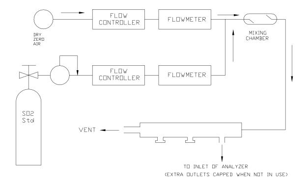
Figure 7-2: Diagram Of Calibration System
