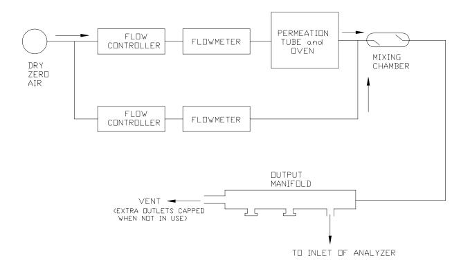
Figure 7-3: Diagram F Permeation Calibration System
