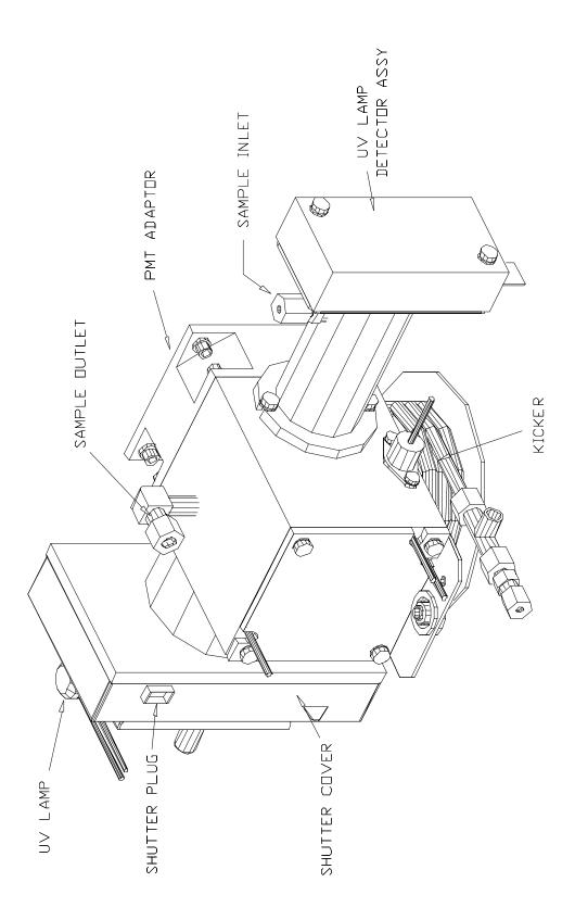
Figure 9-7: SO<sub>2</sub> Sensor Module
