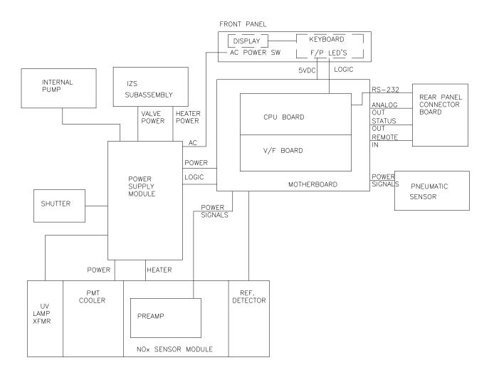
Figure 9-5: Electrical Block Diagram
