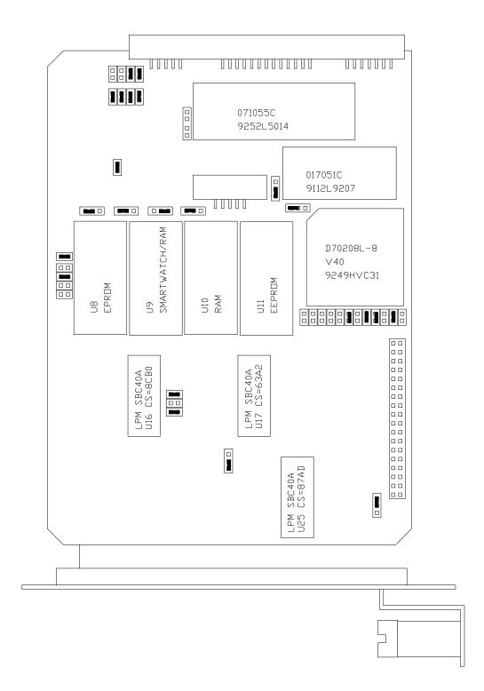
Figure 9-1: CPU Board Jumper Settings
