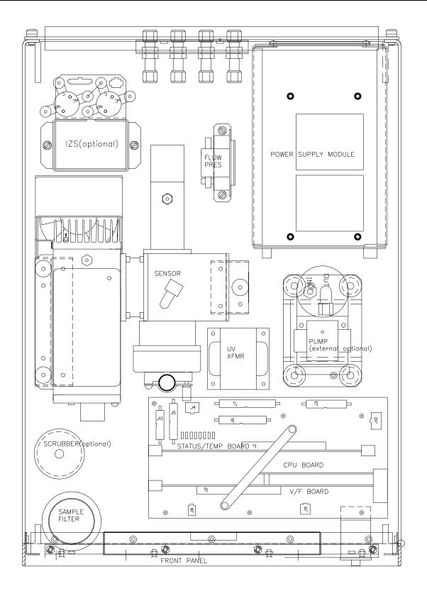
Figure 2-5: Assembly Layout
