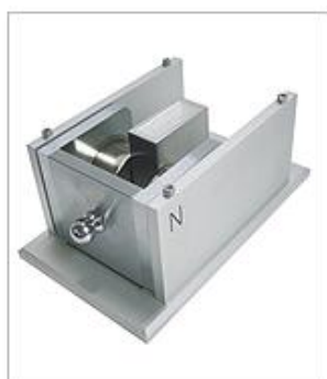
Magnetic flux density input system (0.27T, 0.31T, 0.37T, 0.51T, 1T)
