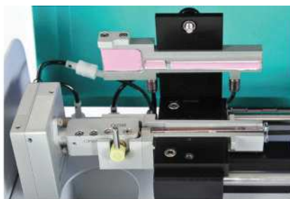
注射器装入检测池，关闭热夹套
