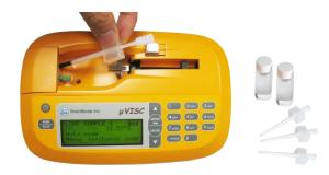
Enter an oil profile, based on reference values. The required values are kinematic viscosities at 40 °C and 100 °C, density at the test condition, and target temperature.
