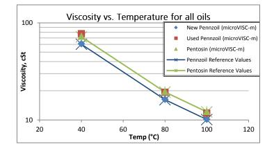
As shown in the preceding tables and graph, *micro*VISC-m could easily differentiate between the two new 5W-30 oils, and detected a large viscosity change between the new oil versus used oil. *micro*VISC-m can generate viscosity data comparable to the output of a viscometer measuring at the actual set point.
