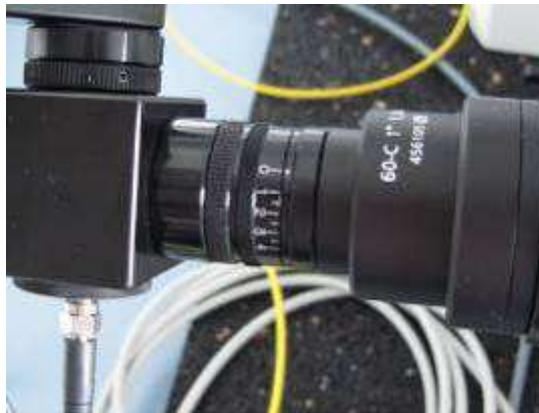
Fig. 6.2.: Iris diaphragm at the detector tube.
