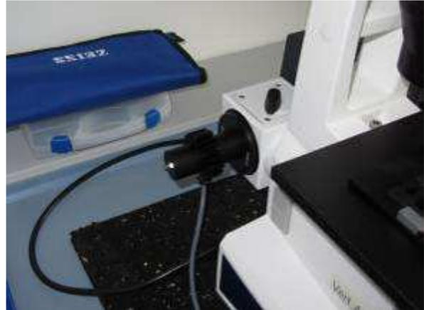
Fig. 5.1, Left: LED Light Source with connection adapter for Zeiss microscope.
