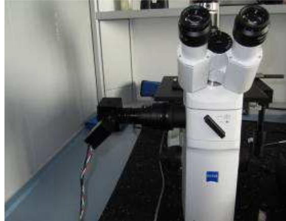
Fig. 5.2, left: OPAL Detector Unit. The detector module is visible in the front.
