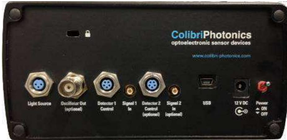
Fig. 3.3: Back side of the OPAL Controller.
