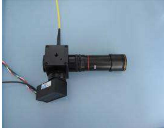
Fig. 3.6: OPAL Detector Unit with ocular adapter.
