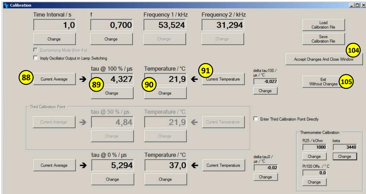
Fig. 7.2.: 1<sup>st</sup> calibration point at air with 20.9% O<sub>2</sub> ( $\Delta$  100%)
