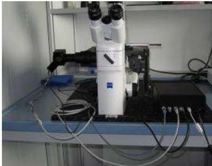
Fig. 5.5., Cable connection of the OPAL Controller to the LED Light Source, the OPAL Detector Unit, computer via USB and power supply.
