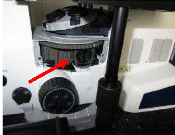
Fig. 5.3 Left: Zeiss filter cube "P&C".
