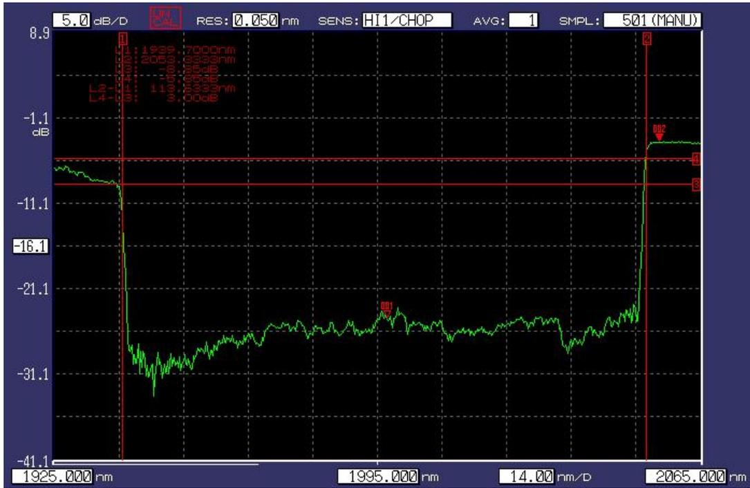
Figure 3. Transmission spectrum of a 2 μm chirped FBG with a bandwidth greater than 100 nm
