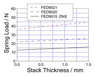
Spring load on stack vs. stack thickness for different springs.
