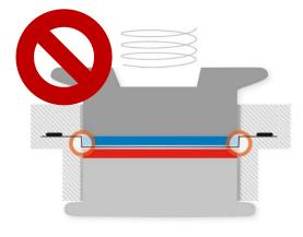
**Gap too large:** Excessive downward bending of built-in separator; reference ring is out of plane with separator.
