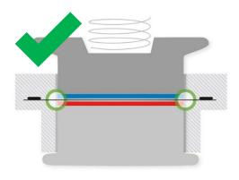
**Good case:** No bending of built-in separator; reference ring is in plane with separator.
