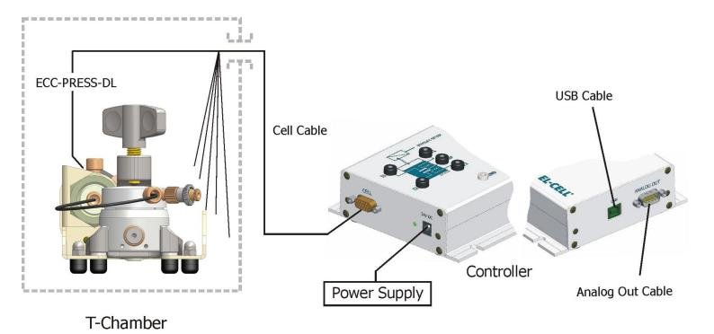
For best results, place the ECC-Press inside a temperature controlled chamber, at a constant temperature between -20 to +70°C. The chamber needs to have a feed-through for cable connection to the controller box outside the chamber.
