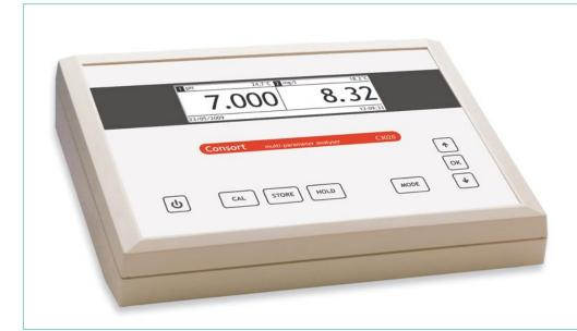
pH: -2...+16 pH ±2000 mV mV: Conductivity: 0...2000 mS/cm Resistivity: 0...200 MΩ.cm Salinity: 0.0...70.0 TDS: 0...100 g/l Dissolved oxygen: 0...60 mg/l
