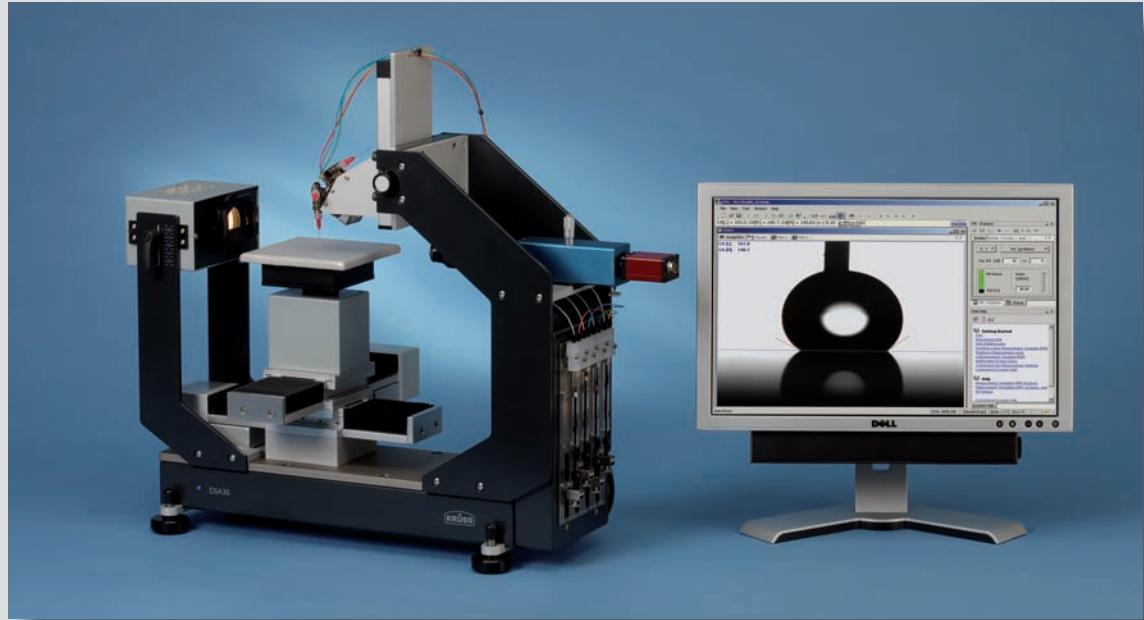
Contact angle – surface free energy – surface tension - roughness: the DSA30 offers numerous possibilities at a competitive price. The modular system provides a wide range of high-performance solutions for studying the surfaces of solids. The contact angle measuring instrument is ideal for QA material testing of medium sized samples at standard measuring throughputs. A large selection of basic components and accessories offers a solution for almost any measuring problem.
