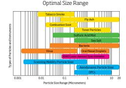
With a size range of 0.09 (90 nm) to 7.5  $\mu m$  this is the right instrument to bridge the 1  $\mu m$  particle size regime, measuring both the accumulation and course particle modes.
