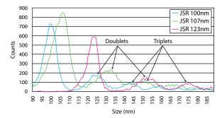
Typical resolution is within 2.5% of the particle diameter at 0.1 µm. The Laser Aerosol Spectrometer can differentiate between 100 nm and 107 nm PSL!
