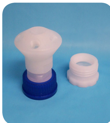
BC-622 6-port manifold for GL45 bottle, with (5) 1/4" NPT ports radially, (1) 1/2" NPT top port Shown with BC-151 thread adapter for GL38 bottle
