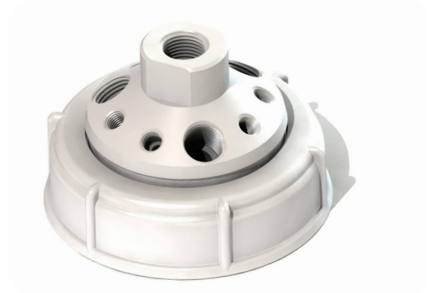
CM-1013 70mm (Hedwin) 10-ported manifold with (6) 1/4-28 ports, (3) 1/4" NPT ports
