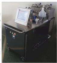
Engineering unit of Sysbiotech Company developed a fully automated Sysbiotech Mobile CIP-station for reactors, vessels and piping, which is currently available in several standard versions with its washing tanks' working volumes of 2x100 L and 2x200 L.
