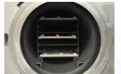
载波系统与水冷式法兰 View on water-cooled flange with carrier system
