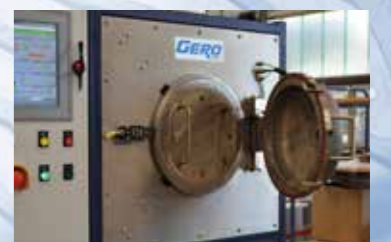
打开门能看到背面的辐射板 Open door with view on backside of radiation sheet package
