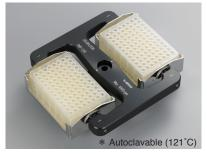
Many researchers want to use microplates so that large numbers of samples can be easily centrifuged using less energy and less time. The 2420 can use the RMP-206 rotor for centrifuging 6 x Micro-plates at 1,790 x g.
