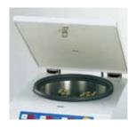
In the event of breakage, all fragments will be safely retained inside the centrifuge unit. Interlocking parts are protected against mechanical impact and employ a two-stage electrical protection circuit.
