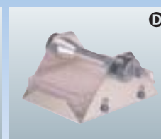
Code No. 053-5170 Eight micro plates can be centrifuged.
