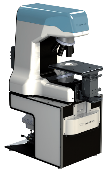
Transmission DHM® combined with a Fluorescence module
