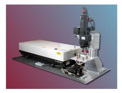
**PLSS-3 Laser Simulation System** is intended for single event effects (SEE) investigations in integrated circuits (ICs) and semiconductor devices (SDs). By varying pulse energy, picosecond laser allows to simulate ionization tracks produced by particles with various linear energy transfer (LET).
