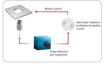
The Nano-Cyte<sup>®</sup> feedback control system. Stabilization is based on the imaging pathway.
