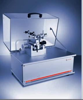
Load: Max.: 60 N Min.: 0.25 N Friction force: up to 20 N
