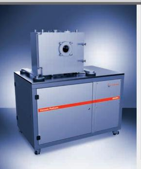
Add any of the instrumented indentation modules inside an enviromental chamber (vacuum, humidity, SEM, ... )
