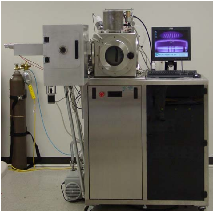
Eight Wafer Cassette Auto Load Un-Load Sputter Up System
