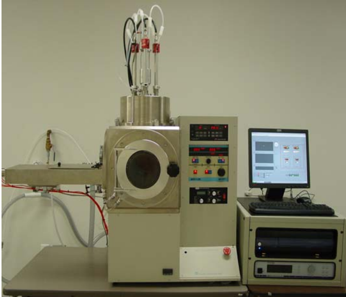
NSC-3000 with Aluminum Chamber and Auto Load Lock
