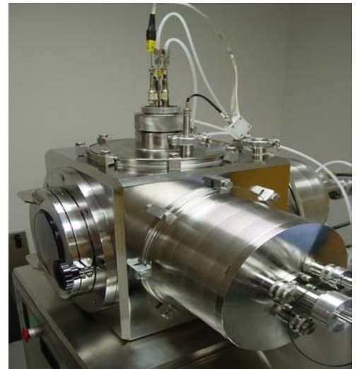
Combinatorial Side Sputtering System with Vertical Platen
