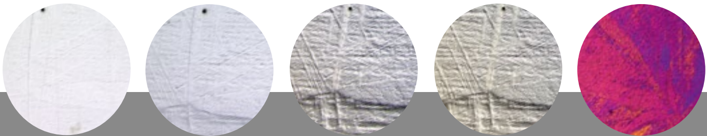
锌：Pl. Fluotar ● 5x BF ● 5x UC-3D ● 5x DIC ● 5x DIC + UC-3D ● 5x Pol. 拉姆达板
