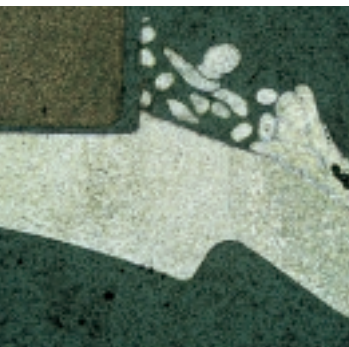
Weld structure, brightfield
