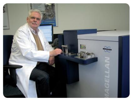
Q8 MAGELLAN covers any application: from primary metal production to metal processing, incoming material testing, etc. From Arsenic to Zirconium, from sub-ppm to percentage levels. Magellan meets complex requirements.
