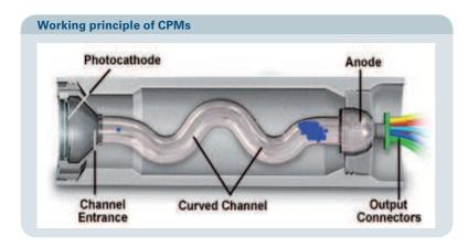
The working principle of a channel photomultiplier. Similar to the classical PMT, but with enhanced properties, photons are converted into electrones and highly multiplied. The reading at the anode gives the light intensity in "digits".
