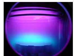
-1000 V DC Bias, 500 °C, ICP On
