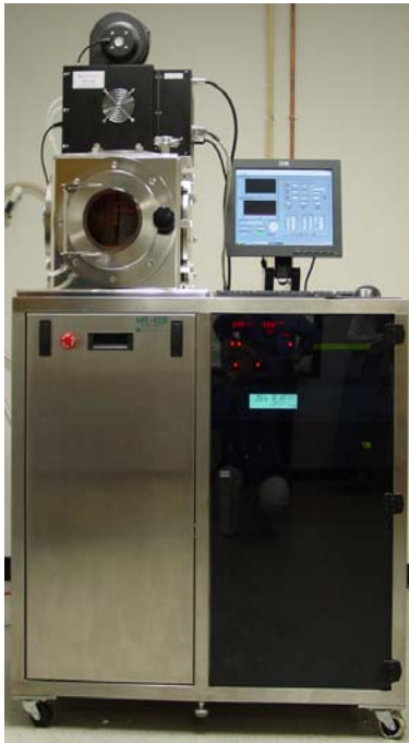
NPE-4000 with ICP Source (Selective Growth of CNT)
