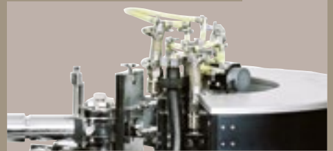
Fixed stage in Debye-Scherrer geometry with monochromator, high temperature attachments and Imaging Plate Detector
