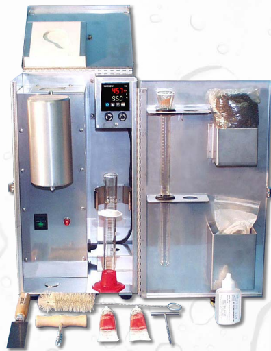
165-14-2: 50 mL Retort Kit, with Electronic Temperature Controller (115 Volt)
