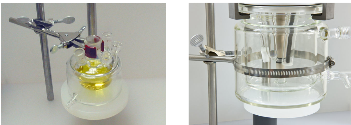
Figure 4.5: Properly Supported and Clamped Electrochemical Cells
