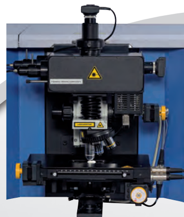
Open-space microscope configuration with DuoScan.
