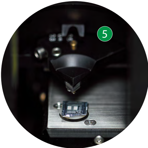
High resonance scanner, auto tip-alignment and tuning
