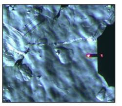
The video optical microscope zooms in to show an HOPG sample surface and the AFM cantilever.
