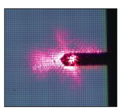
Laser alignment is greatly facilitated with the video optical microscope. This vibrating cantilever is  $250 \mu m$  long. The red spot is from the laser reflecting off the cantilever.
