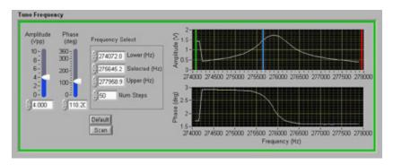
With the window above the resonance frequency of a cantilever is readily measured. Additionally, the phase characteristics of the probe-sample interaction may be captured.
