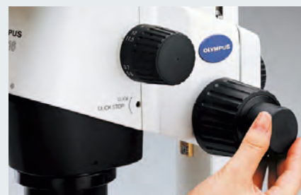
Ergonomic coarse/fine focusing knob
