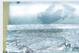
Four-part illumination of surface fracture (metal)
