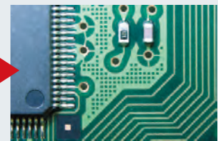
Right-quadrant illumination of PWB
