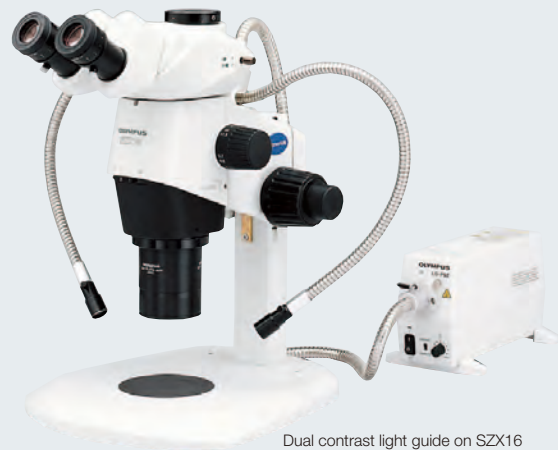
Dual contrast light guide on SZX16
