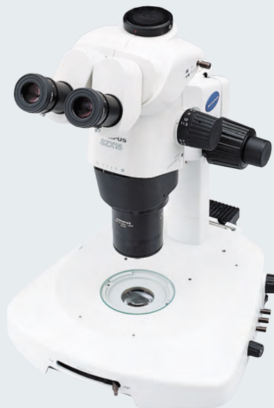
Advanced transmitted light illumination stand (SZX2-ILLB)
