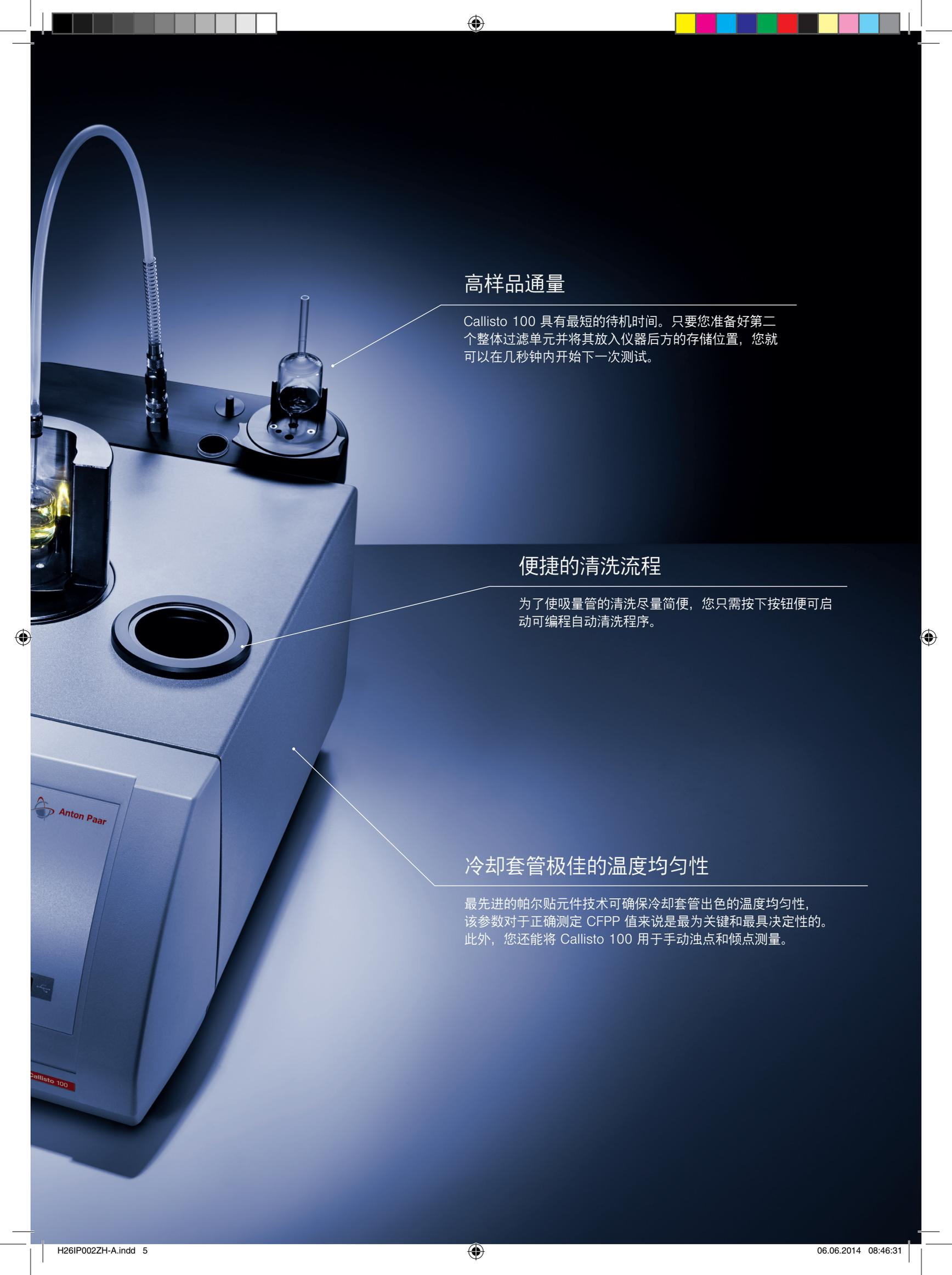
The image shows the Anton Paar Callisto 100 instrument, a laboratory device used for measuring cloud point and pour point. It features a sample chamber, a cooling jacket, and a syringe-like component. The instrument is light blue and has the Anton Paar logo on the front. The background is dark blue with white text and lines pointing to specific features.
