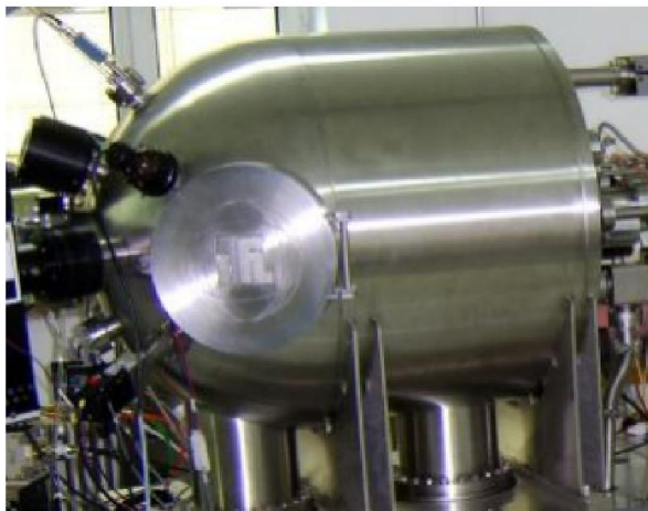
Chamber volume: 0.3 m 3 ; Pumping speed: 1,000 L/s
