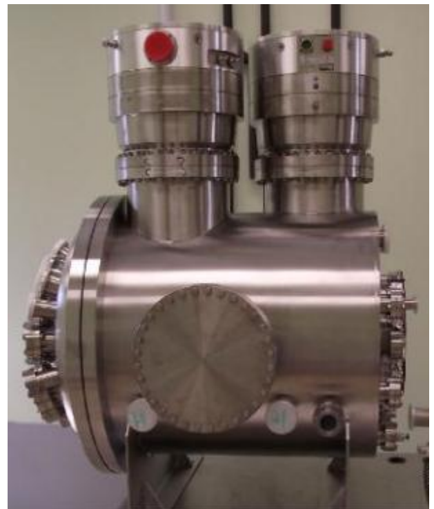
Chamber volume: 0.4 m 3 ; Pumping speed: 4,100 L/s
