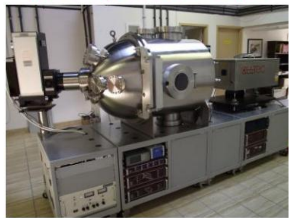
Modern multi-functional LEO space simulator system
