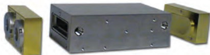
The 5.11m pathlength, 200 mL volume, long path gas cell measures 8\text{-}1/2'' \times 2'' \times 3\text{-}1/2'' , and uses a patented aberration correcting optics for maximum sensitivity.
