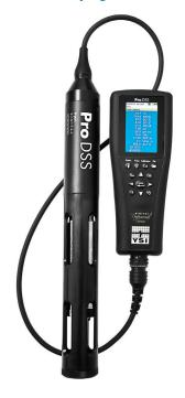
Parameters: Dissolved Oxygen (Optical) **Turbidity** На ORP/Redox Conductivity Specific Conductance Salinity Total Dissolved Solids (TDS) Resistivity Seawater Density Total Suspended Solids (TSS) Depth Ammonium Ammonia Chloride Nitrate
