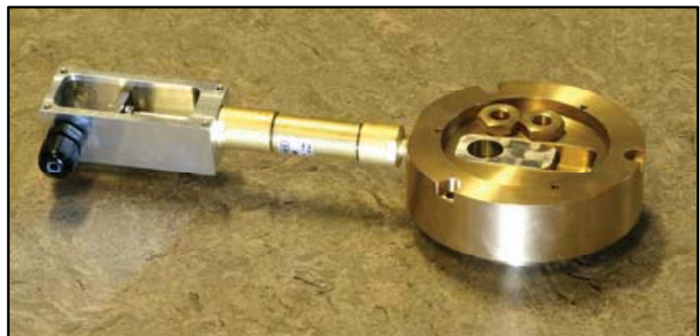
Left: Filament X-ray mounted on a Risø Single grain reader. Right: Shutter for the filament X-ray system.
