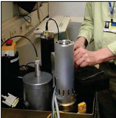
Left: Filament X-ray mounted on a Risø Single grain reader. Right: Shutter for the filament X-ray system.
