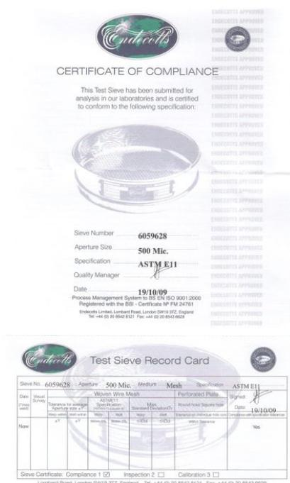
The image shows two documents from Endecotts. The top document is a 'CERTIFICATE OF COMPLIANCE' for sieve number 6059628, with an aperture size of 500 Mic and specification ASTM E11. It includes a photo of the sieve and contact information for Endecotts Limited. The bottom document is a 'Test Sieve Record Card' for the same sieve, providing detailed measurement data for woven wire mesh and perforated plate, including aperture size, mesh, and inspection dates.
