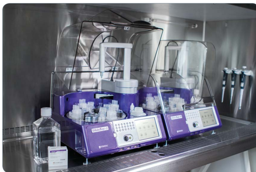
Figure 2. The compact design of the RoboSep™-S allows multiple units to be placed side-by-side in a biological safety cabinet.
