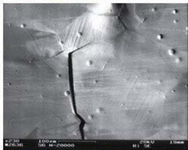
5'100 N Compression Load 390 \mu\text{m} Displacement
